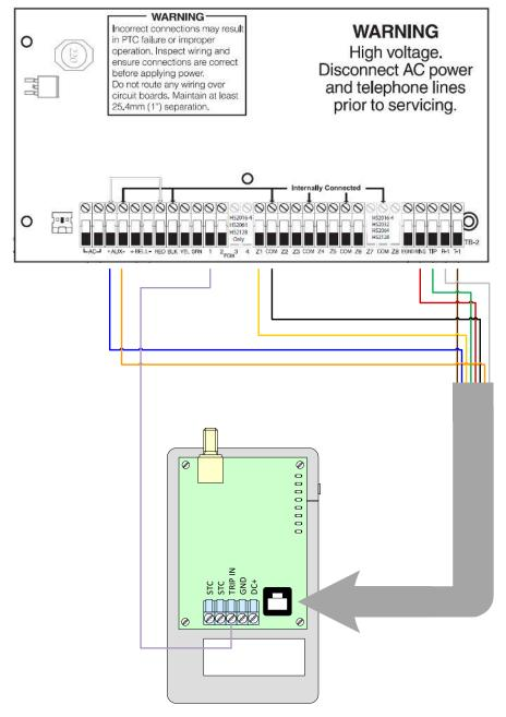
**Note:** Although a resistor is not depicted here, one may be required by the Keyswitch zone in accordance to the Panel's specifications. For more information, please refer to the Panel's Installation and/or Programming Manuals.
