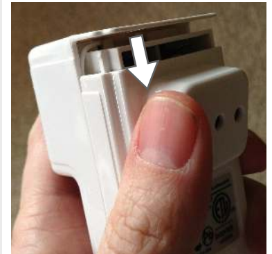
Slide back cover of the casing downward and remove from device
