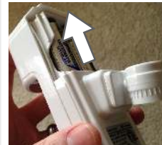
Align back cover and slide upward to secure on device
