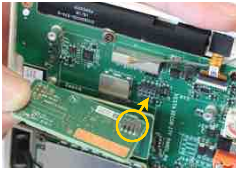
Match the pins on the bottom of the IQ Card-IS to the terminal on the IQ Panel
