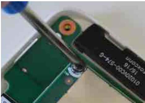
Install and tighten the provided locking screw to secure the IQ Card-IS into place.
