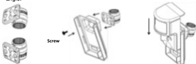
Mounting Arm Orientation (Top: Teeth Up, Bottom: Teeth Down) Attach Mounting Arm to Sensor-Back Attach Sensor to Sensor-Back
