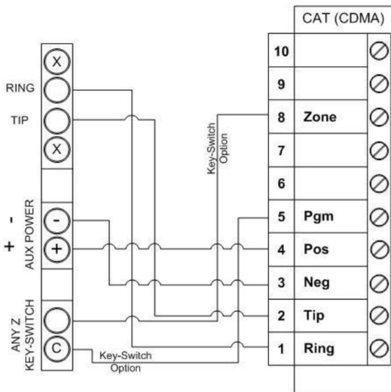
GE Control Wiring & Key-Switch Option
